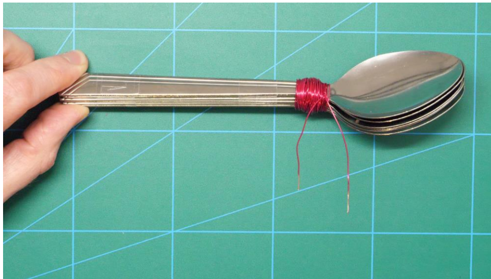
Fig. 1. The hand wound inductor comprises a length of enamel-insulated copper wire wrapped 80 times around a stainless steel core that was formed
